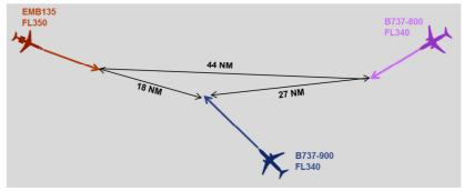
The heading instructions are meant to maintain the predicted horizontal separation of over 5 NM between the EMB135 and the Boeing 737-900, while "to be level in 2 minutes" instruction is issued to ensure that the EMB135 is below the B737-800 before the horizontal separation is lost.
