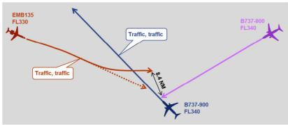
As both aircraft are "locked" on their headings there is no loss of separation. Soon after receiving the TA, the EMB135 stops its descent and reports "unable rate due to TCAS TA".
