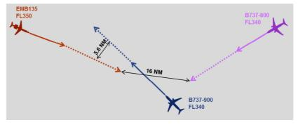
After 45 seconds, when the EMB135 is passing through FL348, both the EMB135 and B737-900 get TAs against each other. The TAs are issued because the aircraft are slightly converging and the time to Closest Point of Approach falls within the TA generation threshold.
