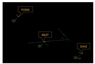
Figure 1 – 1655:28 - indicated levels are FL – add 270ft for altitude
