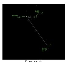
Figure 2: No1 F15 loss of Mode C data.
