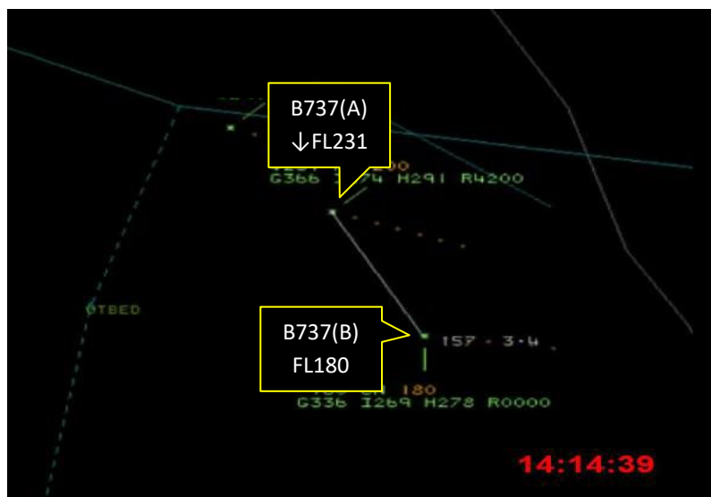
Figure 1. Relative positions of event aircraft when [B737(B)] was transferred to Doncaster ATC.
